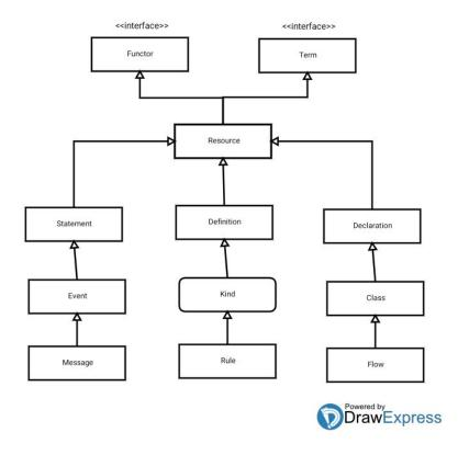
All hierarchy classes (including Functor and Term interfaces) are defined in terms of RDF Quads. Each Quad instance context aggregates other Quads instance contexts according their meaning.
