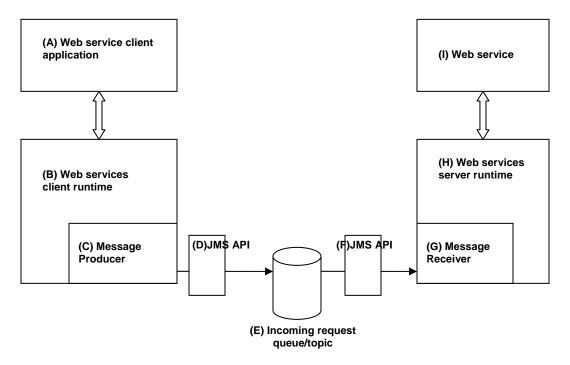
We have a web services client application (A) that is supported by the vendor's client runtime (B), which contains the message producer (C). The message producer (C) uses the JMS API (D) to create and deliver request messages to the request queue or topic (E). On the server side, the message receiver (G) is contained in the vendor's server runtime (H) and receives the request message from the request queue/topic (E) and processes it by using the JMS API (F).
